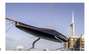
and 11-man crew clear of the water. Many questioned whether it was technically possible to balance a single-hulled boat of this size with no keel on just two hydrofoils.
