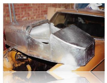
The chassis was welded up using one inch square mild steel tube with the body being pop riveted in position, then the hard part trying to find wheels and tyres to fit. In those days, without the likes of eBay, it took some time to come up with the wheels. Eventually I found two brand new wheel barrow wheels (not quite what I wanted but needs must), then I had to order the other two and wait weeks for them to arrive.
