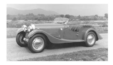
Coincident with the demise of the Plus 4, 2020 marks the 70th anniversary of the Plus 4. The Plus 4 at its introduction in 1950, was fitted with a 2088cc Standard Vanguard engine installed on a strengthened 4/4 chassis with a wheelbase lengthened by 4 in (102 mm). Hydraulic brakes, at first all drum, were fitted for the first time on a Morgan.
