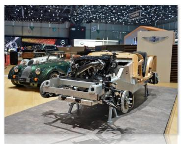
architecture. The all-new CX-Generation bonded aluminium platform has been designed and developed in-house and is introduced with intention for use in future premium Morgan models throughout the next decade.
