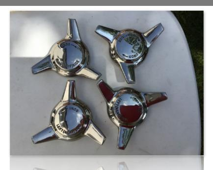
Set of 4 off 3 eared spinners 8 TPI (Threads Per Inch) for MGB and others (?). All MG's up to 1964 including early MGB's had 12 TPI. The 8 TPI will fit all later B's, midgets, sprites and MGC's and most Morgans! good condition. £.100.
