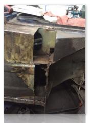
work on the offside wing which had some rather draughty rust holes in it. I managed to patch and lead load the deep damage and use Ultimate filler in the areas that only need a light skim. Hopefully the finished product will provide a good base for the paint finish.
