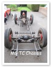
2012. We could now see how a "T" series car became EX175 - the design of the TC chassis is very similar to that of the MGA, though the latter had a widened chassis to allow the driver to sit within the chassis rather than above it.
