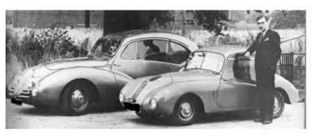
produced in Coventry around an ash frame fabricated by a local boat-builder.
