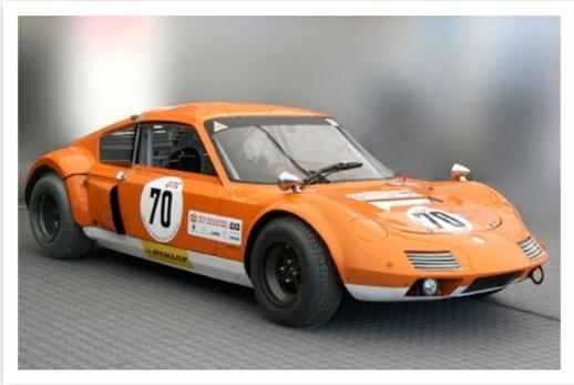
One last development under Trojan in 1964 was the Elva GT160, a BMW engined car designed by Trevor Frost. Weighting only 11cwt, this would have been a real flier. Only three prototypes were built before it was considered too costly to continue.
